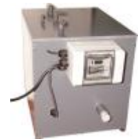
Figure 27 Drain water pump
