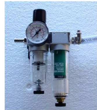
Figure 31 Compressed air filter
