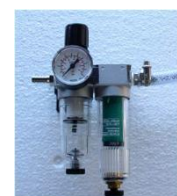
Figure 29 Water and oil filter for compressed air
