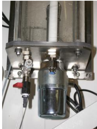
Figure 47 Heater housing located below the humidifier
