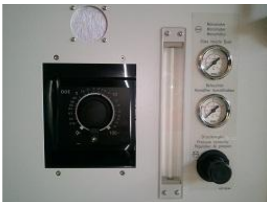
Figure 33 Air pressure control on the control panel
