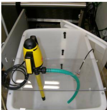
Figure 81 Reservoir with circulation pump
